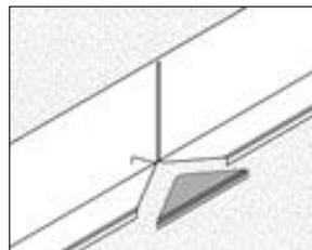
**STEP 1** - Cut down the vertical wall (not to the very top) and cut away a V in the shoulder foot (at least 120 degrees) on the side where you will bend it in.
