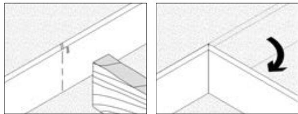
**STEP 1** - Score a line down the back of the edge and create a sufficient opening (5-7mm) in the double folded lip at the top.
