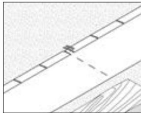
**STEP 1** - Score a line down the back of the edge and create a sufficient opening (5-7mm) in the double folded lip at the top.
