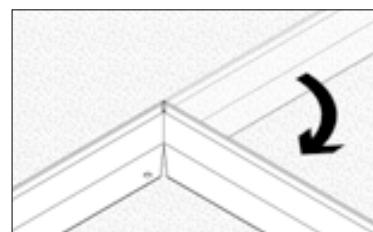
STEP 2 - Bend by hand (past the 90 then back for right angles) and perfect shape with rubber mallet.
