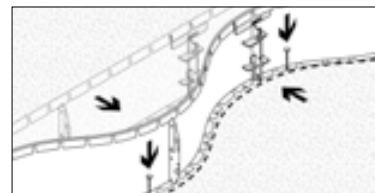
STEP 6 - Set these two edges upright and flex to position where desired, use fixing spikes as temporary placeholders.
